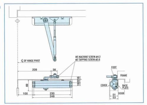
◆Parallel Application (with Flat Parallel Bracket) D-2580SMP
